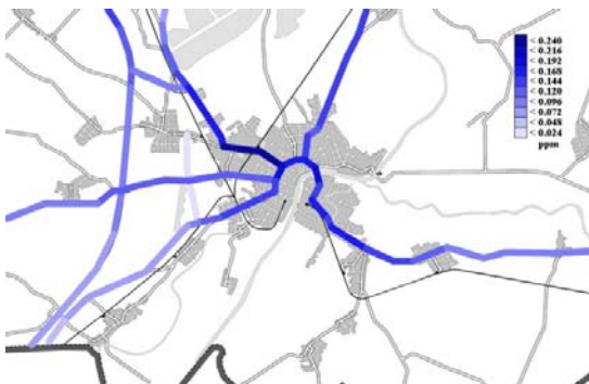
Fig. 8a. Annual mean NO 2 concentrations on the major roads of the Szeged region, 2006, ppm ( h = 1 m).
