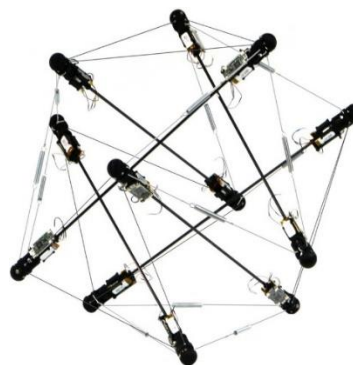
Fig. 4. Robot proiectat cu ajutorul conceptului tensegrity IcoTens (Columbia University- Fivat ș. a. https://www.creativemachineslab.com/tensegrity.html#:~:text=Tensegrities%20are%20structures%20made%20out,used%20frequently%20in%20architectural%20design. )
